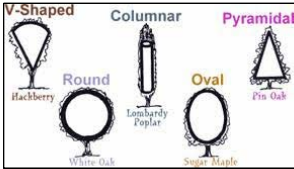
Figure 15 – V-Shaped trees (such as Eucalyptus) are generally preferred as they offer the greatest screening where antennas are mounted. The tree species shall be selected based on surroundings and ideally placed in a grove.
