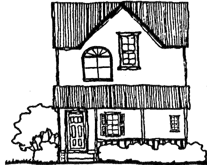
Architectural elements are out of balance and window styles are incompatible
