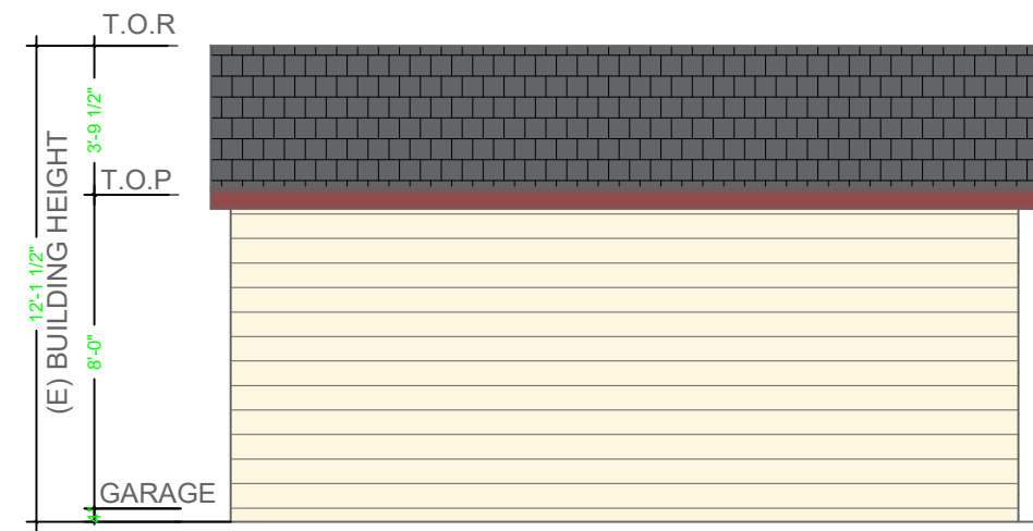
(E) GARAGE WEST ELEVATION
